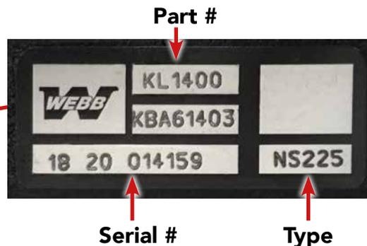
After a long life in service or while still on the vehicle it can be difficult to read the information on the ID plate. Therefore the following can be useful in assisting identification.
